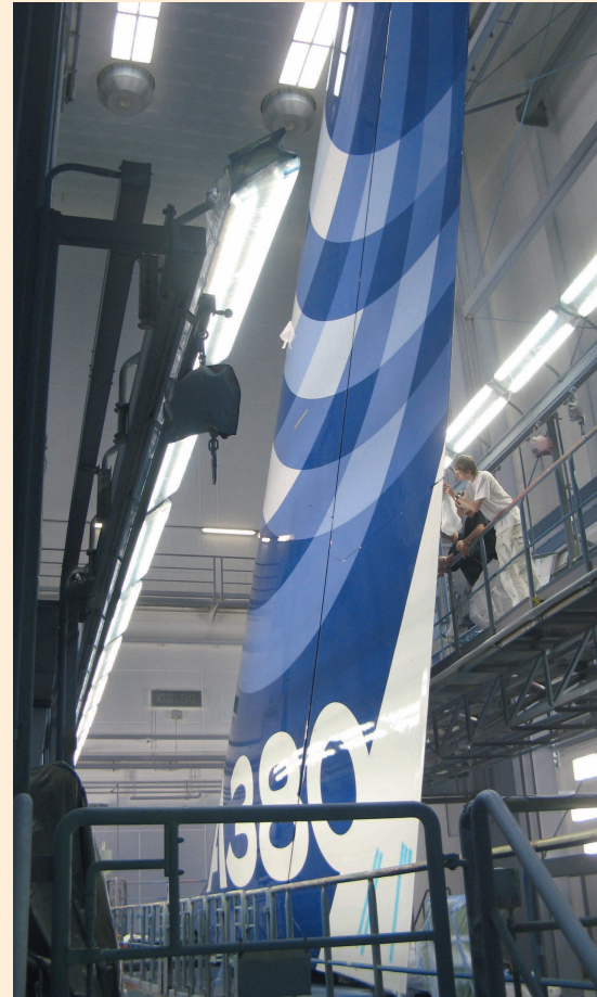
Tall tails: The A380 tail comprises a substantial amount of composite material
