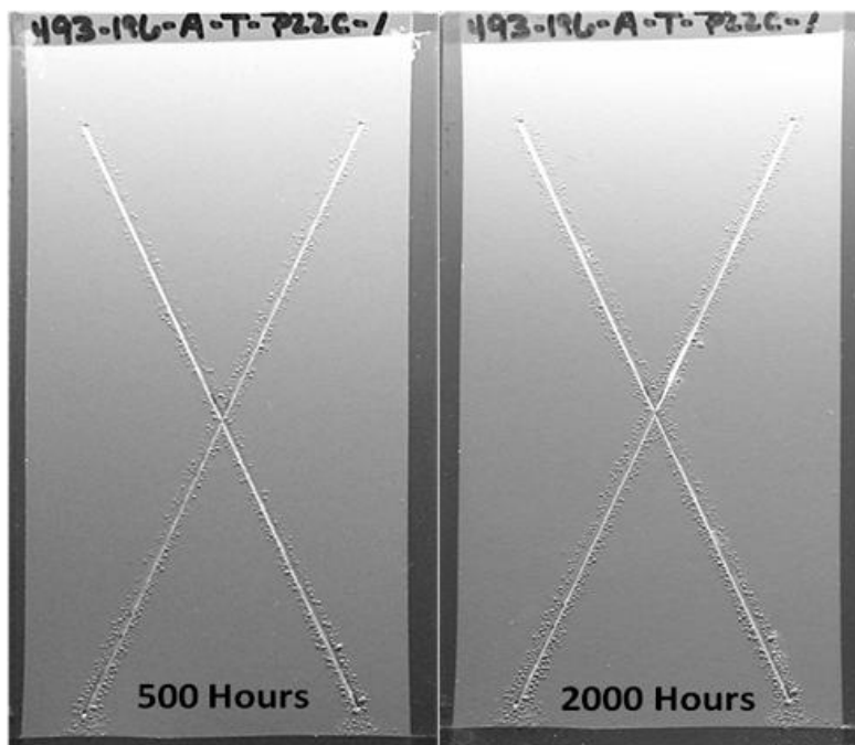
FIGURE 5 - Performance of early prototype in NSS, clad 2024-T3
